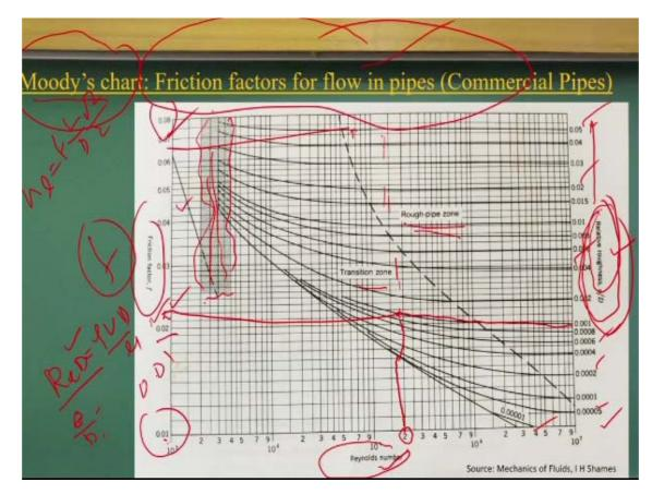
Now this Moody chart compiles for conducting series of experiment in using commercial pipes or artificially roughened pipe. So again plotting with the Reynolds numbers and the friction factors. This side is friction factors. Again I am writing f equal to
