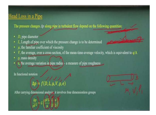
Now let us now what we are doing it first the dimensional analysis. So if there is a pressure drop along a pipe in a turbulent flow depends upon the following quantities. Pipe diameters, length of the pipe okay diameters, the length of the pipe  $\mu$  is similar to the coefficient of viscosity, familiar to the coefficient of viscosity and average velocity rho and the small e represents the average variations in pipe radius.
