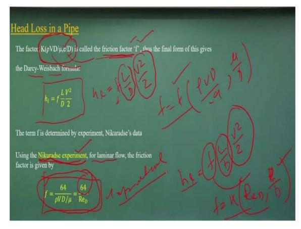
This is new definitions we put it that this constant, it is not a constant, it varies with respect to the Reynolds numbers with respect to the ratio of roughness height and the diameters which we call a constant, the friction factors. Because for particular flow systems, you know the Reynolds numbers for a particular pipe, the type of the pipes, we know this the roughness height and the D.
